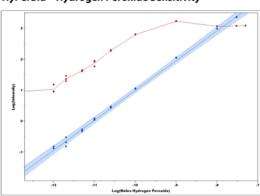
Three replicates of 50  $\mu$ L serial dilution of Urea Peroxide (Aldrich) were prepared in deionized water and added to a white 96 well plate. 50  $\mu$ L of Lumigen HyPerBlu reagent were added to each well. The intensity was measured using a Lumistar Optima (BMG). 50  $\mu$ L of Amplex Red (Life Technologies ) were tested with a second set of replicates on a Flouroscan Ascent (Labsystems). Readings at the 24 minute time point are reported.
